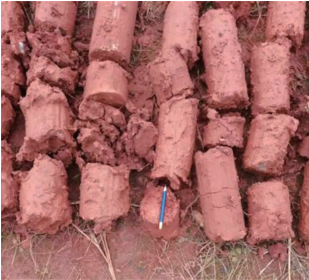
图 6 ZK4 钻孔揭露滑动面 Fig. 6 Exposed sliding surface by ZK4 borehole
