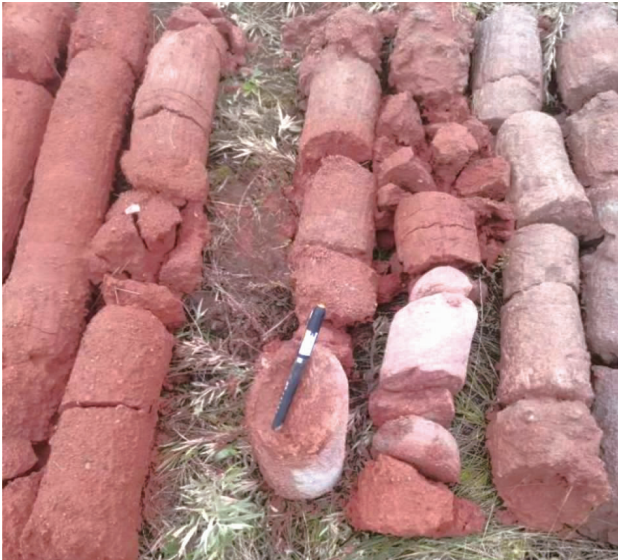
图 5 ZK3 钻孔揭露滑动面 Fig. 5 Exposed sliding surface by ZK3 borehole
